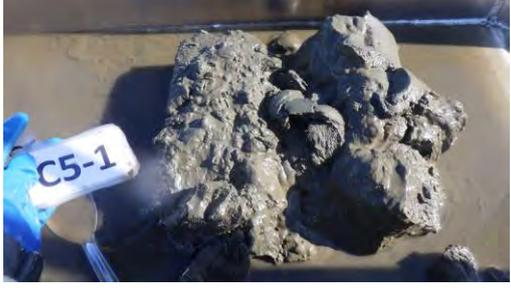
A photograph showing a sample of dark, silty sediment in a white tray. A white label with the text "C5-1" is held by a blue-gloved hand to the left of the sample. |
